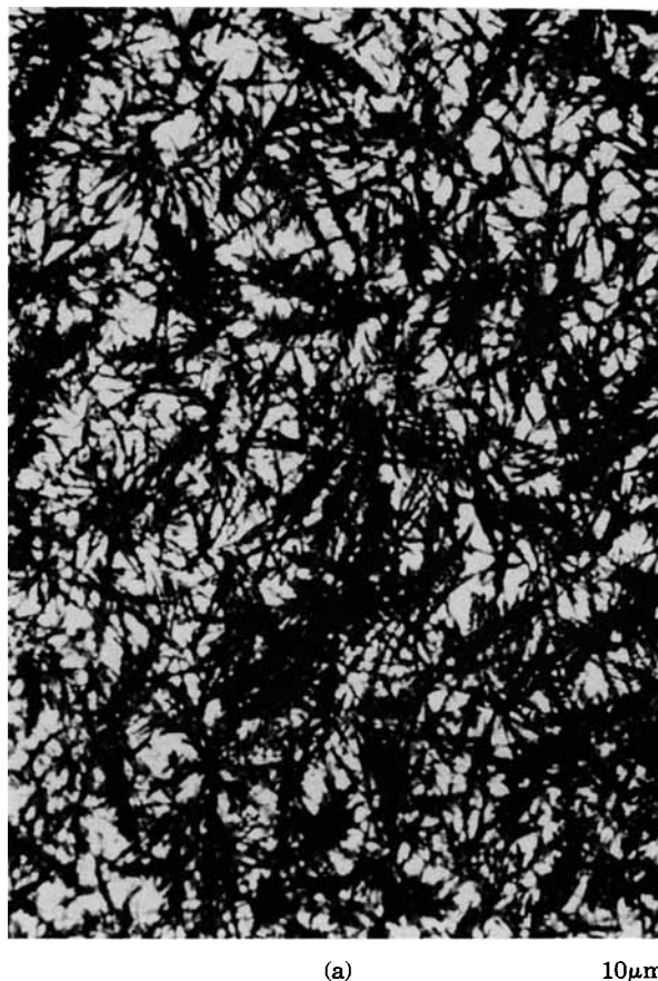
Fig. 4. Micrographs of polystyrene (a) and polyvinylchloride (b) films containing 3 wt% of the TCNQ salt 16.
